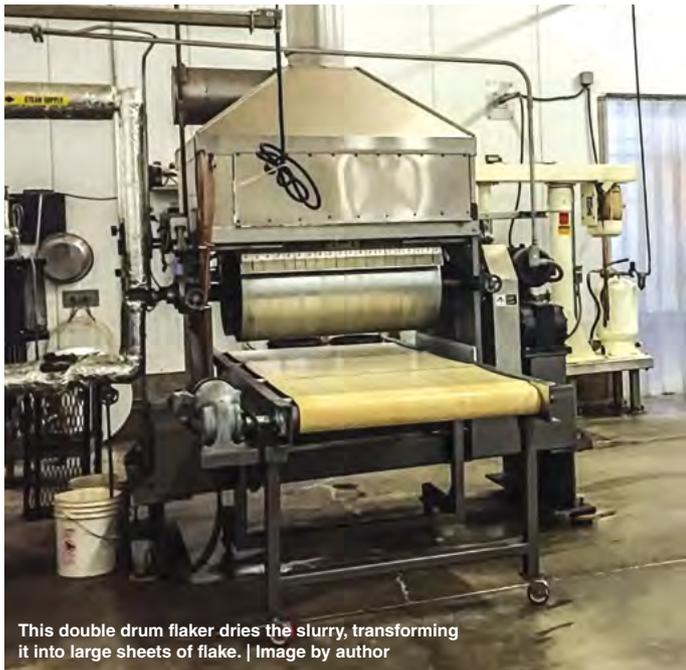
This double drum flaker dries the slurry, transforming it into large sheets of flake. | Image by author
